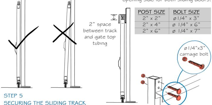
The stopper block is **welded** inside the sliding track at 8 1/2" from the gate opening. Two more stopper blocks will be welded on the top of the door frame. One Flush to the gate opening and the second will varie with the door size. **You must secure both**
